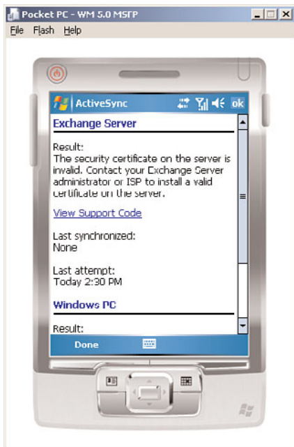
FIGURE 23.6 Error received when Windows Mobile device does not trust the root of the CA.
